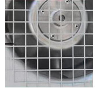
Air inlet safety net
